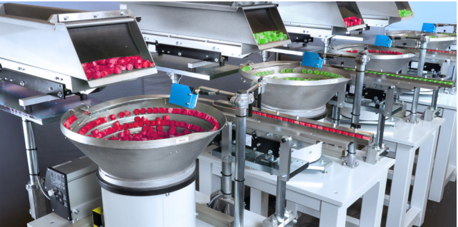
Typical application: SRC-N 250 with KSB-ZA 250 feeder bowl of grade 1.4301 material
