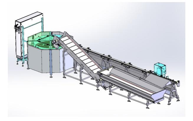
RNA's VariFeed<sup>™</sup> is a high-speed, automated feeding system for handling chocolate and cereal bars. Up to 400 products per minute can be sorted for the subsequent packaging process. Meeting high food grade standards, the modular system can be designed for multiple products and customer layouts.
