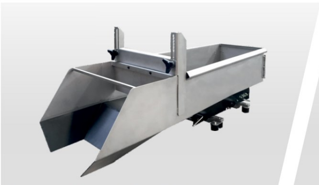
Vibrating hopper with a quick emptying flap
