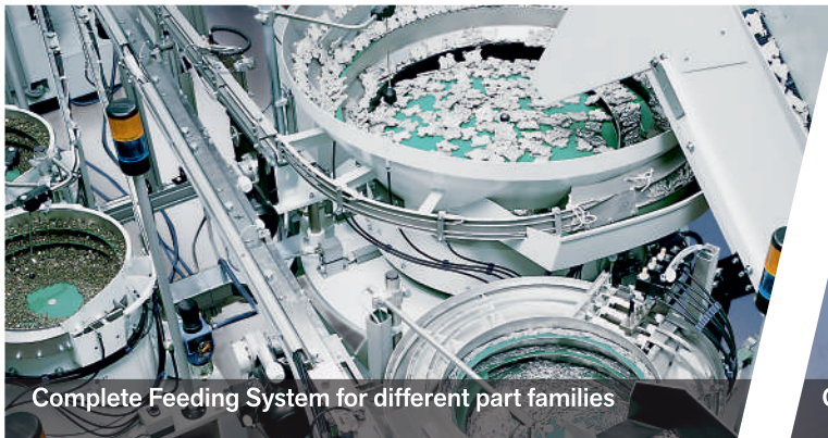
Linear Feeding System with a SLF 1000-1000 with Control Unit ESM 3000-16 (ill. right) & SLL 400-800 with Photoelectric Fork Sensor and Control Unit ESM 3000-16
