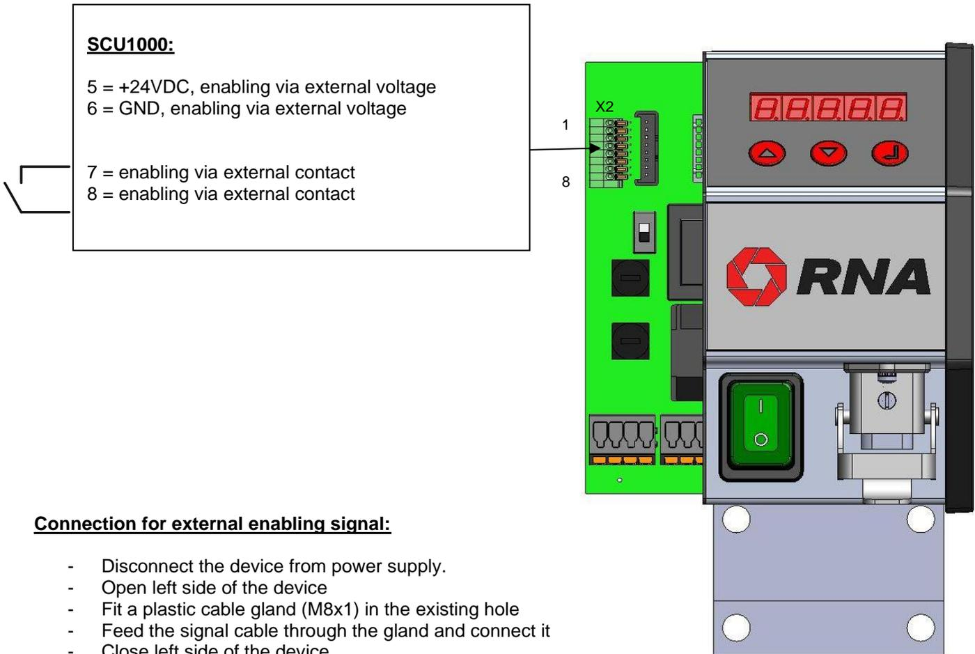
**Connection for external enabling signal:**
