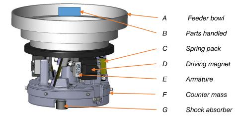
Driving magnet D is rigidly connected to counter mass F. When the driving magnet is energized it exerts a force on armature E. This force is transmitted to bowl A mounted on spring packs C, causing the bowl to vibrate. The angle of the spring packs defines the direction of bowl movement.
