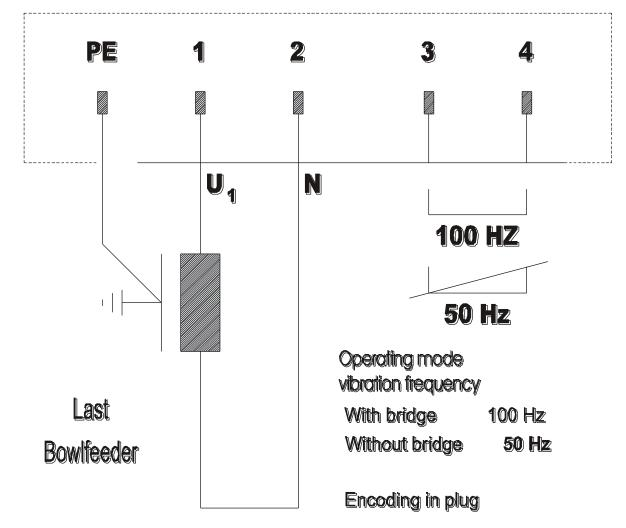
With jumper: The jumper must be inserted between connections 3 + 4.
