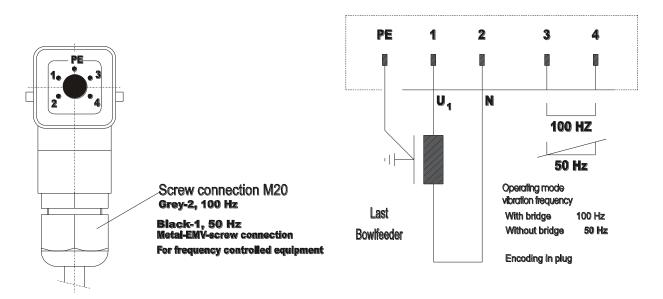
The bridge has to be installed in connection 3+4
