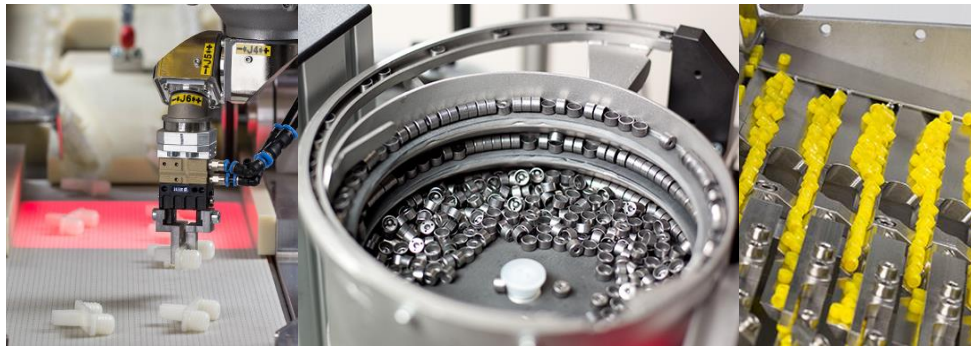
Sorting and Feeding of Plugs for Non-reusable Syringes
