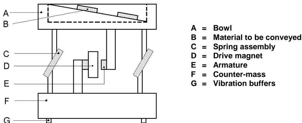
The drive magnet D is firmly connected with the counter-mass F. When current passes the drive magnet, it exerts power on armature E. The power is transmitted to bowl A, which is supported by the spring assembly C. The moving direction of the bowl is determined by the angle of the spring assemblies.
