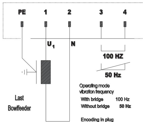
The bridge has to be installed in connection 3+4
