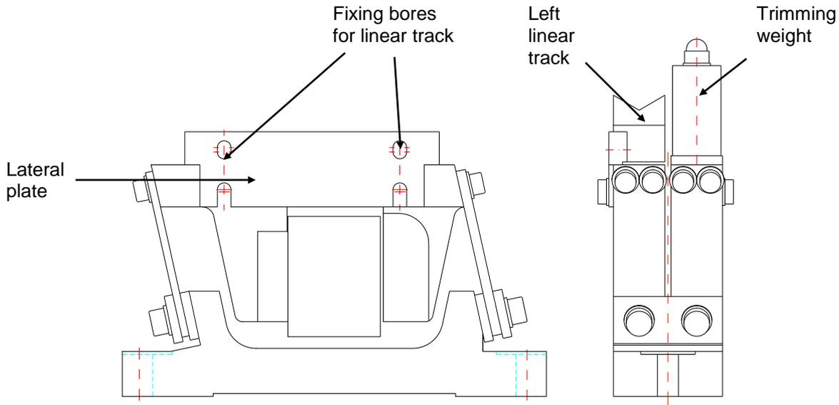
The vibrating sections are designed with recesses on the outer side to receive the angle brackets and trimming weights. The runout height of the linear track can be precisely adjusted during initial installation by means of the slot-type bores in the lateral plates. Thus no track readjustment is necessary when the linear track is removed and reinstalled for cleaning purposes or change to a different product.
