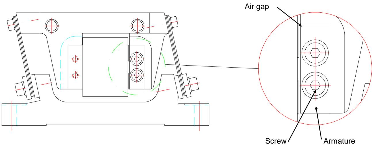
**Table 5: Setting values for the air gap between armature and magnet core**
