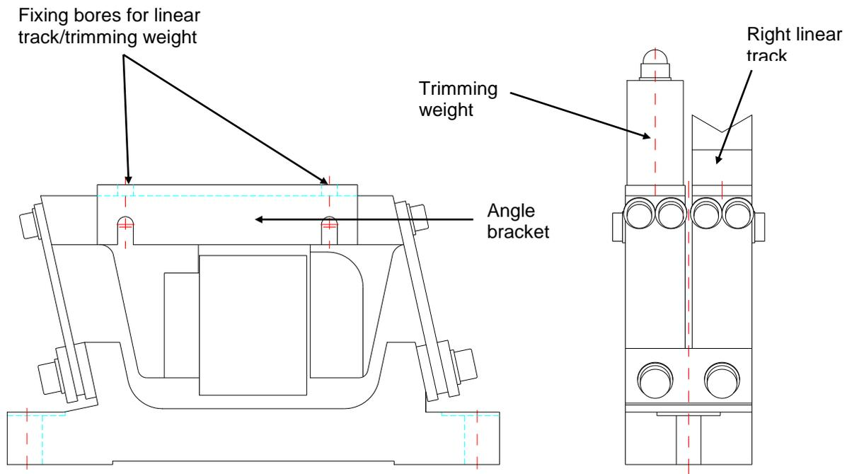
**Figure 5:** Linear track mounted with lateral plate
