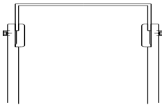
Figure 7: Mounting the sheet metal belt frame
