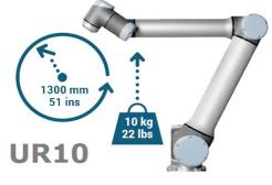
experience. The robot can be programmed by simply moving the robot arm to desired waypoints or touching the arrow keys on the easy-to-use touchscreen tablet.
