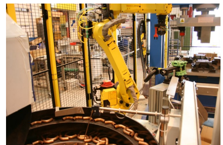
<< Vision Guided Robot picks up fittings from a bowl feeder and loads them into a free issue press
