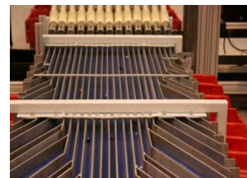
<< Out-feed conveyors fitted with separation lanes to transport the parts into tote bins
