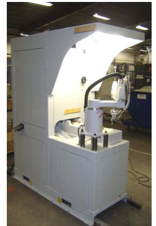
MicroFlex equipment with Epson 4-axis Scara robot
