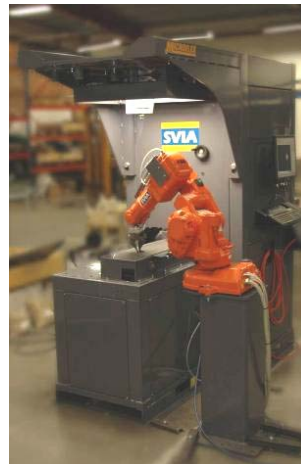
MicroFlex equipment with ABB 140T robot
