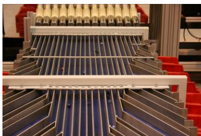
>> Out-feed conveyors fitted with separation lanes to transport the parts into tote bins
