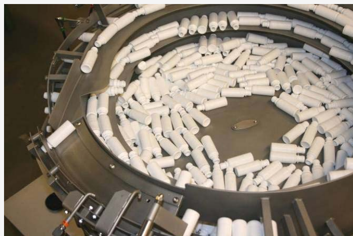
▲ RNA Quick Release system feeding 3 sizes of plastic pharmaceutical bottles
