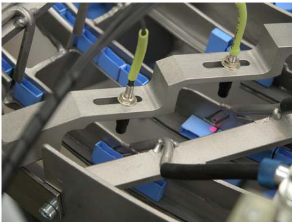
Orientation-Recognition with Proximity Switches. Post-sorting.
