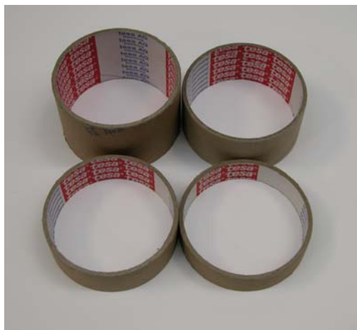
Cardboard Shells, 8 Types Ø76.2 mm, Height 9 – 50 mm
